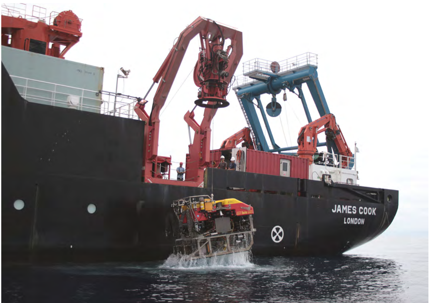
Recovering the Isis deep water Remotely Operated Vehicle (ROV)
