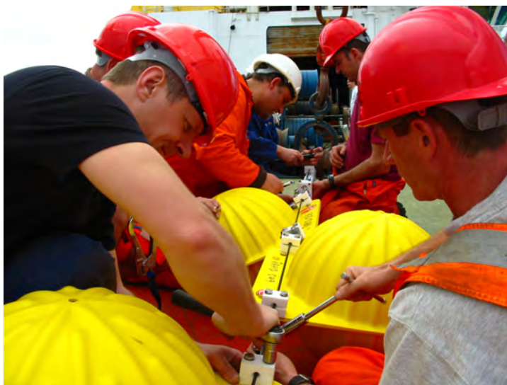
Preparing a mooring for deployment
