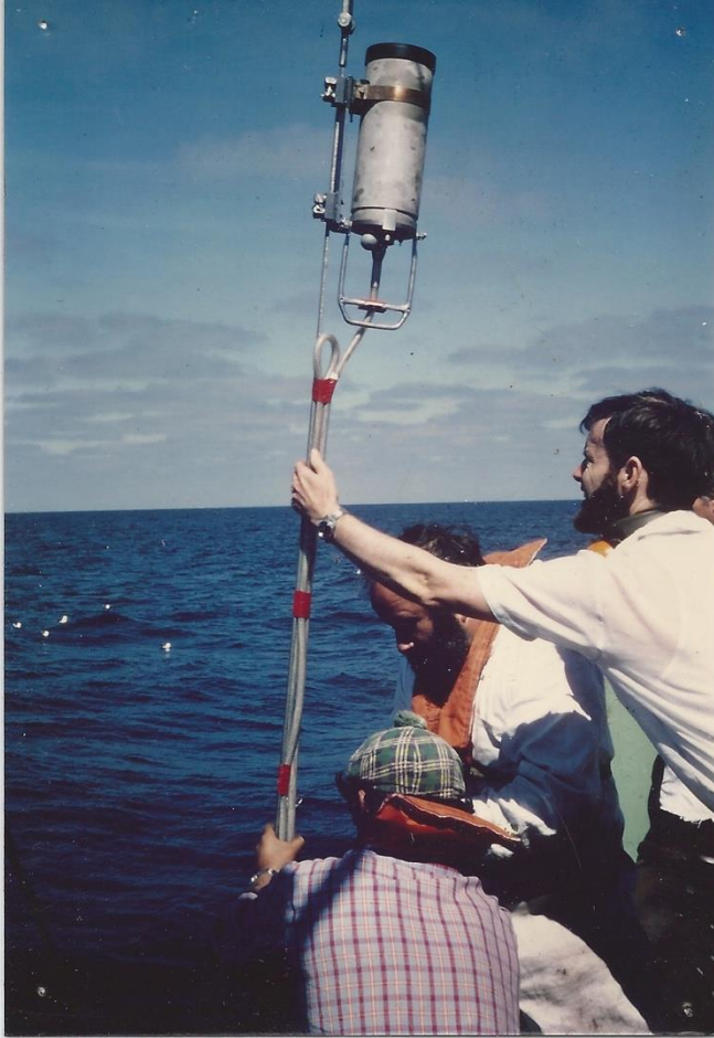
Raymond attaching a thermistor chain to the wire on RRS Discovery cruise D86 in September 1977.
